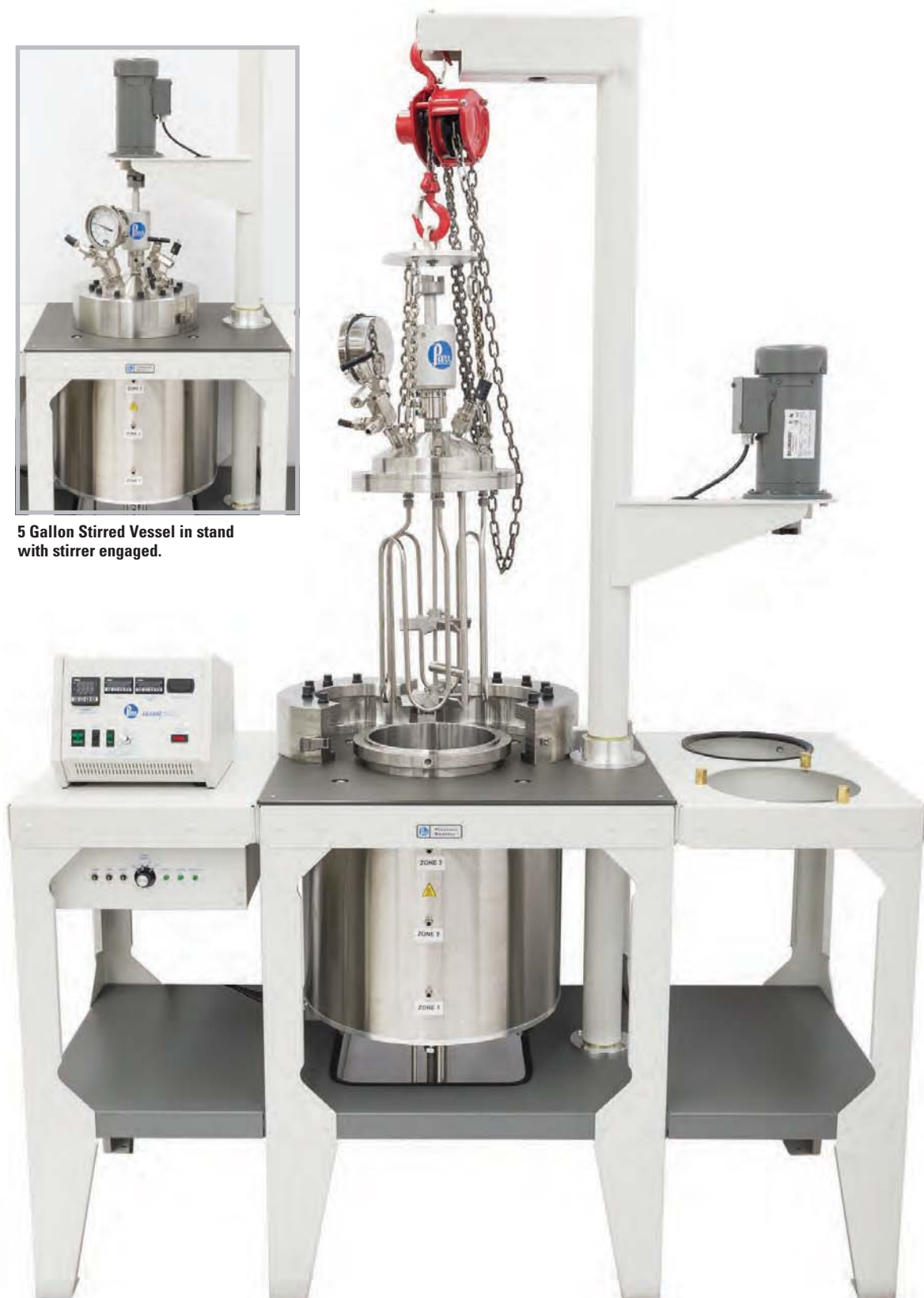
4555 Table Floor Stand Reactor, 5 Gallon Moveable Vessel with Head removed from Vessel, Manual Hoist, and a 4848M Controller.
