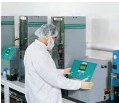
Carver Auto "C" presses molding medical components.*
